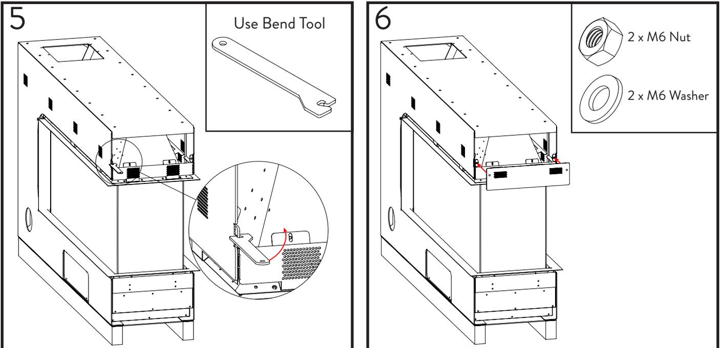
Use the supplied bend tool to bend the tabs on the top front of each side. Affix the front panel in place at the top. Use the supplied #8 - 5/8 screws to affix the KWU onto the fire (2 screws per side).
