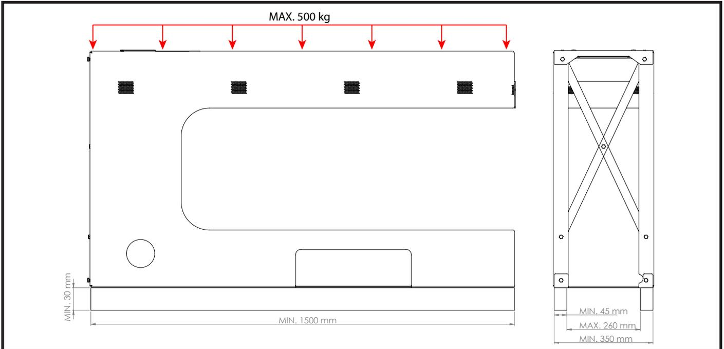
The KWU will need to be attached to timber framing with the dimension shown above (not supplied). Begin by setting the bottom on the timber. Set the left and right sides on top and affix using the 16 x #8-1 1/4 screws.
