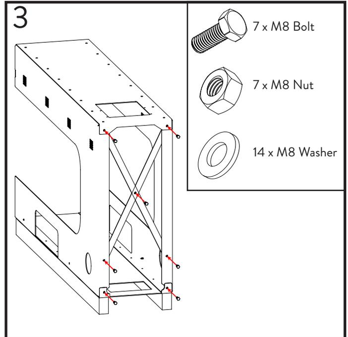
Set the top onto the two sides and affix. Attach the 2 x hangers as cross braces across the back. Slide the KS1150 Peninsula or KS1150 LH or RH Corner into the KWU. The holes on each side are to assist with access while sliding the fire in.
