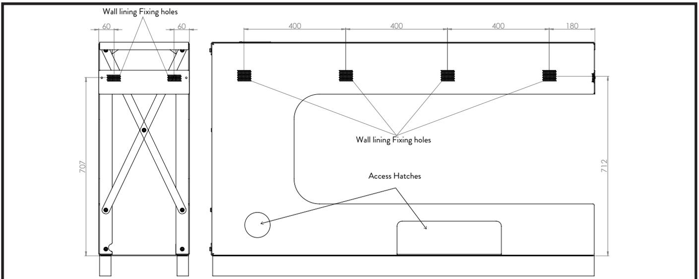
The wall lining fixing holes in the top of the KWU can be used for fixing plasterboard or wall cladding with either screws or construction adhesive glue. The access panels may be clad over; they do not need to remain accessible for service.
