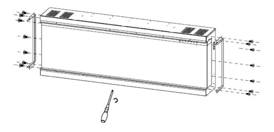
4. Remove the screws from the fireplace as shown in the picture below.
