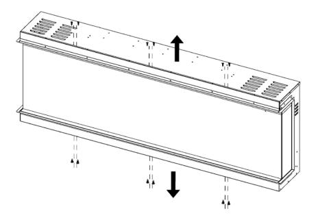
5. Fix the brackets with the screws in the previous step.
