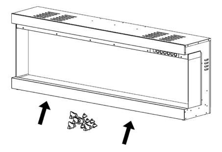
4. After placing the decorative crystals or pebble, fasten screws back on the glass panel.
