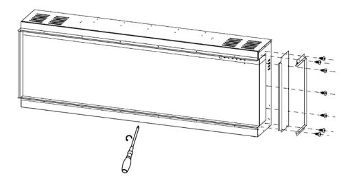
3. Fix back the fending bar after the panel is removed.
