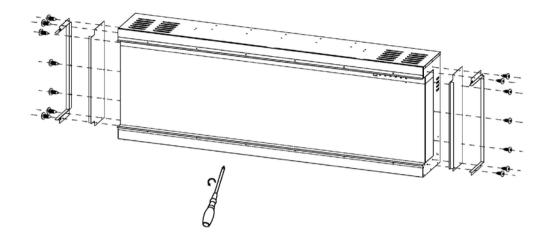
3. Fix back the fending bars after the panels are removed.
