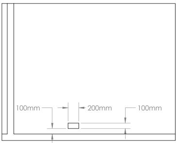
AN AIR VENT OR VENTS ARE REQUIRED ON THE REAR OF THE ENCLOSURE AND MUST BE VENTED TO OUTSIDE AIR. THE BOTTOM EDGE OF THE LOWER VENT OR VENTS MUST BE NO MORE THAN 100mm ABOVE THE FLOOR AND HAVE A MINIMUM SURFACE AREA OF 20,000 SQ mm E.G. 200 X 100mm. THE MESHED VENT MUST BE KEPT CLEAR AT ALL TIMES AND VERMIN PROOFED.
