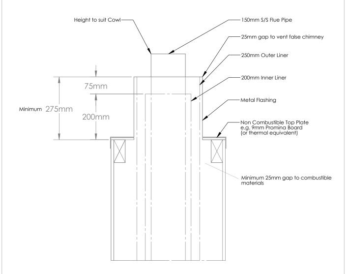
NOTE: IT IS VERY IMPORTANT THAT THE SPACE BETWEEN THE FLUE PIPE, INNER CASING AND OUTER CASING ARE VENTED AT THE TOP.
