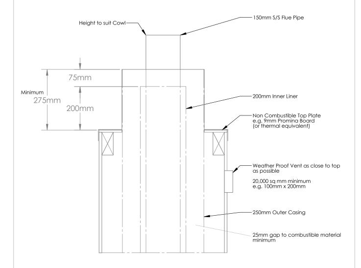
NOTE: IT IS VERY IMPORTANT THAT THE SPACE BETWEEN THE FLUE PIPE, INNER CASING AND OUTER CASING ARE VENTED AT THE TOP.
