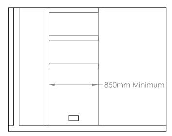
FRAMING REQUIREMENTS AS PER NZS:3604 (SHOWING MINIMUM REQUIREMENTS)
