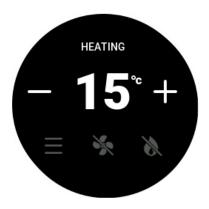
Note: Before starting up, the appliance has a 15 to 30-second pre-ignition purge. During this time, a fan runs by itself before attempting to ignite. A visual indicator on the top of the remote screen shows which part of the startup process the appliance is in (see above).
