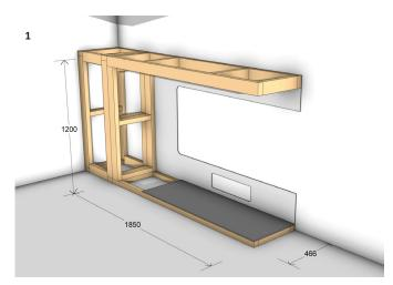
Build the chimney framework with consideration to flue pathways. The minimum cavity opening dimensions should be as above. Construct the KWU framework to the dimensions over page and fit the rear panel. Ensure a continuous base for the fireplace.
