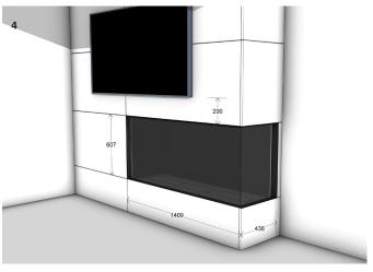
Attach wall linings to the framework and and KWU, maintaining a 3mm gap from the fireplace trim. Follow the provided wall lining cutout dimensions above. Complete the project by adding additional finishes or fixtures.
