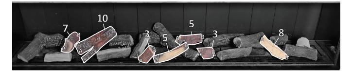
NOTE: Place a single layer of ember rocks on the infill and burners. Improper positioning of any fuelbed media may create carbon build-up and will alter the unit's performance. Malfunctions due to improper fuel media placement will not be covered under warranty
