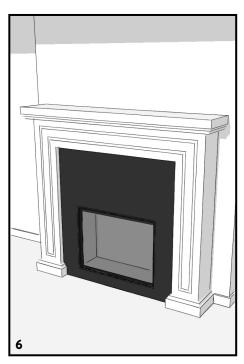
Fit the mantel surround to the wall and fix in place. Complete the project with any fixtures or finishes. A hearth is not required.
