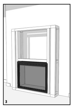
Fit the frameless brackets to all 4 sides of the viewing area. Install the appliance into the framed cavity. Minimum appliance cavity dimensions are 676mm W x 570mm H x 350mm D. The appliance base is 55mm of floor level.
