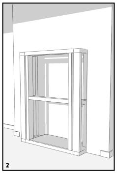
Provide additional framing to support the mantel surround and infill panel. The maximum mantel surround framing is 1320mm W x 1277mm H x 166mm D
