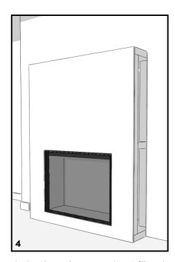
Apply a 10mm substrate to pack out infill panel. This can be a combustible or non-combustible board. The cut-out dimension will be 30mm larger than the infill panel: **672mm W x 515mm H**
