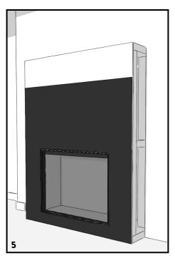
Fix the custom infill panel\* to the substrate with adhesive. The infill panel cut-out dimension is: **642mm W x 485mm H.** This will leave a **3mm** gap to the frameless finish brackets on the appliance.
