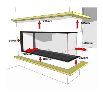
Ensure all clearances are met to any combustible or heat sensitive materials in front, above, to the side, or below the fireplace viewing area. Following these clearances, will allow the use of standard building materials, whether combustible or noncombustible. To reduce these clearances, use non-combustible materials.
