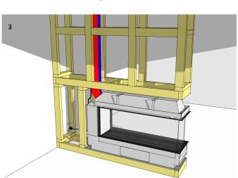
Install electrical, network connections, and gas supply.
