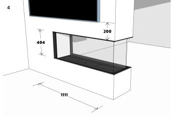
Attach wall linings to the framework and fireplace, maintaining a 5mm gap from the fireplace trim. Follow the provided wall lining cutout dimensions above. Complete the project by adding additional finishes or fixtures.
