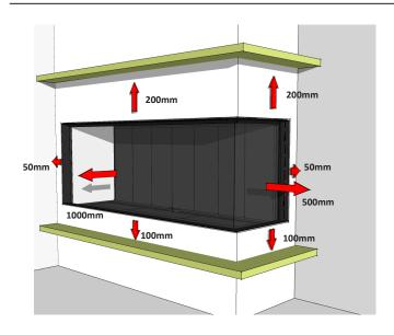
Ensure all clearances are met to any combustible or heat sensitive materials in front. above, to the side, or below the fireplace viewing area. Following these clearances, will allow the use of standard building materials, whether combustible or noncombustible. To reduce these clearances, use non-combustible materials.
