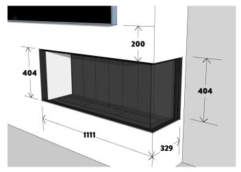
Attach wall linings to the framework and fireplace, maintaining a 5mm gap from the fireplace trim. Follow the provided wall lining cutout dimensions above. Complete the project by adding additional finishes or fixtures.
