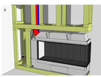
Install electrical, network connections, and gas supply.
