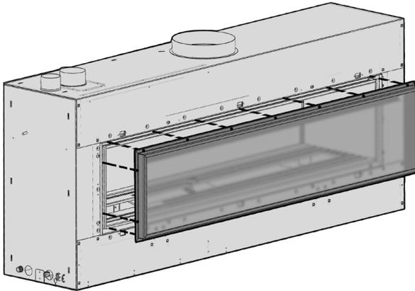
Pull the top of the frame toward you slightly and lift the glass and frame out and away from the fire. Place the glass & frame carefully aside.
