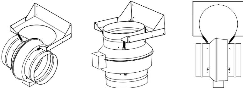
**NOTE: The duct fan must be installed in a location accessible for service or replacement; a service hatch (to allow for access) may be required.**
