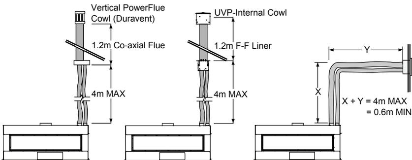
*NOTE: You must provide sufficient access to the powerflue to enable it to be serviced in the future. This means that the fan unit must have sufficient access to allow it to be replaced if necessary.*
