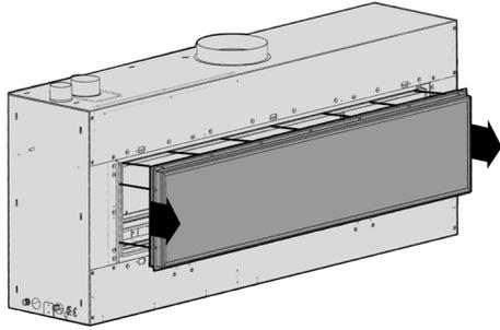
3. Screw the wall lining trim brackets on to the appliance chassis as shown in photo.
