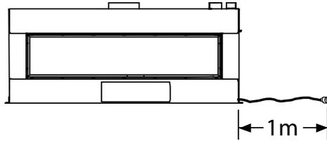
This connection **must** be accessible after the heater has been fully installed so that the appliance can be safely disconnected from the mains power supply prior to servicing.
