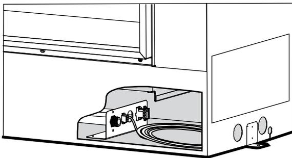
If you do not wish to connect the fireplace to the modem, the Network / Ethernet cable should be run to somewhere accessible by a service technician, such as a cupboard.
