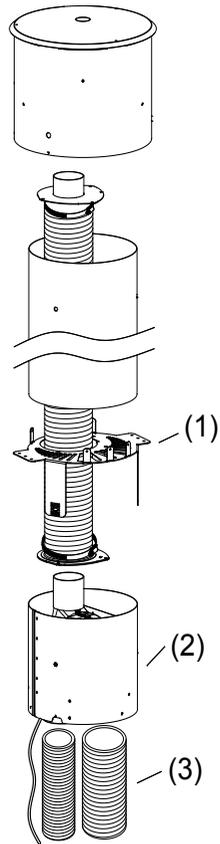
**NOTE: The UVP-Internal and the flexi flue connections must be installed in a location accessible for service or replacement; a service hatch or removable flashing to allow access is required.**
