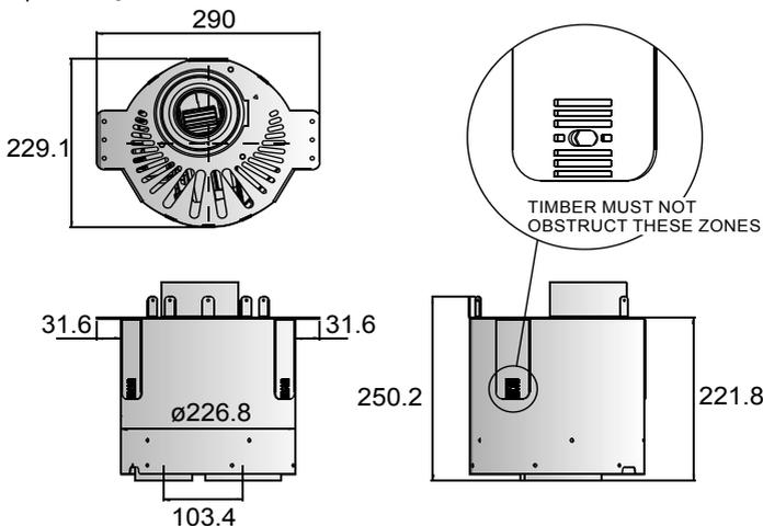
The UVP-Internal kit is intended for use within an accessible roof space or 'chimney' construction.
