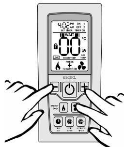
Now hold down the ‘EDIT TIMER’ and ‘ACTIVATE TIMER’ buttons simultaneously; the remote display will show the current configuration of either ‘NG’ for Natural Gas or ‘LP’ for ULPG/Propane. To change this configuration, hold down the ‘EDIT TIMER’ and ‘ACTIVATE TIMER’ buttons simultaneously for 5 seconds. This will now have toggled between gas types.
