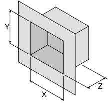
Ideal Hole/Cavity Size for Horizontal Powerflue
