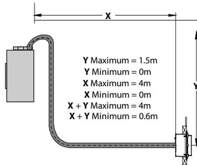
***NOTE: All sections of horizontal flue, if flexible, must be sloped back toward the fire at a rate of no less than 20mm per metre, to allow any condensation to run back into the appliance.***
