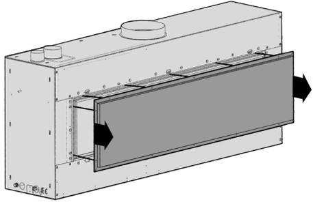
2. Unscrew the firebox rear panel and remove it. Sometimes extra force may be required to remove this panel as the sealing tape can 'glue' itself to the painted surface.
