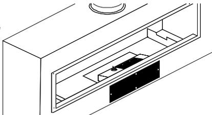
Turn on the gas. Turn the power on. Check the inlet pressure upstream of the appliance using the test point installed earlier.
