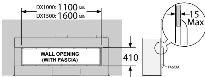
A 15mm or less wall lining must be used when installing a DX-series fireplace with a bevelled fascia, as this is the maximum distance the bevelled fascia can sit off the front face of the fire, as shown. For wall linings of a total thickness of 10mm or larger, a “Linear Trim for Bevelled Fascia” may be purchased to cover any exposed wall lining.
