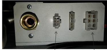
If the fans are not plugged in, it will result in an error when starting the appliance.
