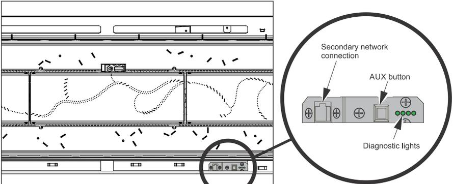
To access the auxiliary on/off button, remove the bottom trim bracket by lifting the bracket upwards (shaded grey in the diagram below).
