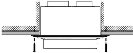
B) By attaching the optional wall terminal installation brackets to the sides of the cavity and attaching the horizontal powerflue wall terminal to these, from the front:
