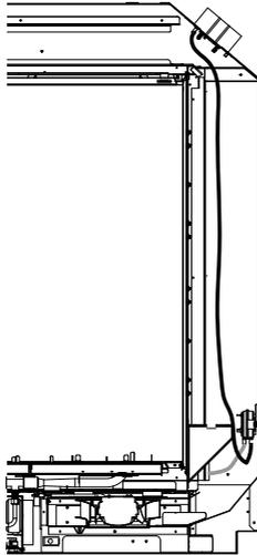
When reconnecting the pressure switch, be sure to connect the tubes as shown in the diagram below. The black tube should be connected between the grey side of the pressure switch and the low pressure port. The translucent tube should be connected between the black side of the pressure
