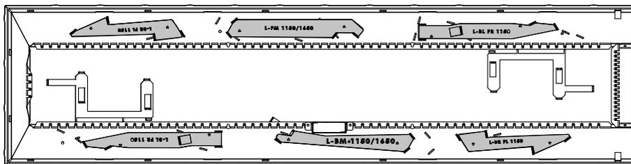
Attach all retainers by feeding the tabs from the **UNDERSIDE (unpainted side)** through the cutouts on the infill. Fix each retainer in place from the top of the infill with the screws provided.
