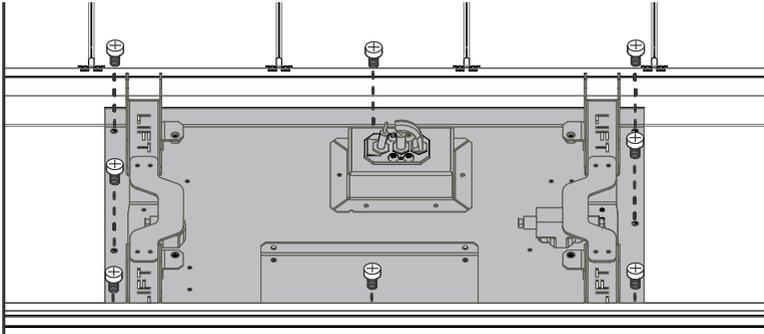
Remove the 'engine' by lifting up and to the right. This is still connected internally to the gas hose and power cables.
