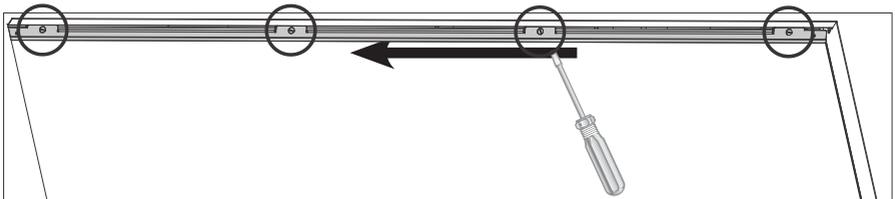
**NOTE:** When replacing the glass, check the channel that the glass sits in for debris that may be sitting on top of the fiberglass tape. Remove any debris prior to placing the glass. If you feel resistance when leaning the glass towards the fireplace, remove it and double check for debris in the glass channel.
