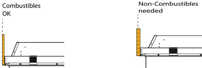
**Note: The wall lining directly above the appliance will get warm and hence may discolour paint finishes that are susceptible to temperature damage. The heat may also distort vinyl wall coverings. For durability of finishes and surfaces you should contact the relevant manufacturer for their specification and avoid materials with temperature ratings not suitable for use above a fireplace (see section A2 on page 6).**
