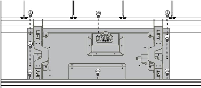
Remove the 'engine' by lifting up and to the right. This is still connected internally to the gas hose and power cables.
