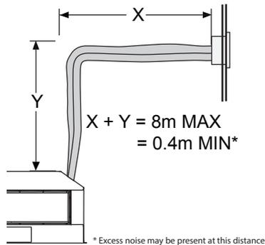
*Note: When flueing above the fire, the pipe must slope towards fire - NOT towards the terminal. Also when flueing below the fire, the pipe must slope towards the terminal - NOT towards the fire.*
