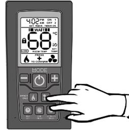
The high setting for the currently set gas type is displayed first (indicated in the clock segments at the top). Pressing the plus or minus keys will change the setting up or down respectively, which will change the gas pressure measured at point A or D. The large digits will blink rapidly after the setting is made until the verification is received from the fire.
