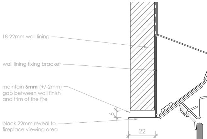
*Note: a 20mm or less wall lining must be used when installing a KS1150 Peninsula 400 fireplace. A 10mm wall lining is recommended for ease of installation.*
