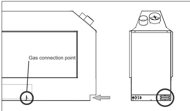
Access for connecting the gas supply to the gas connection point (shown in the diagram above) should be through the access hatches located on the front and back of the appliance (the front as shaded in the diagram below).
