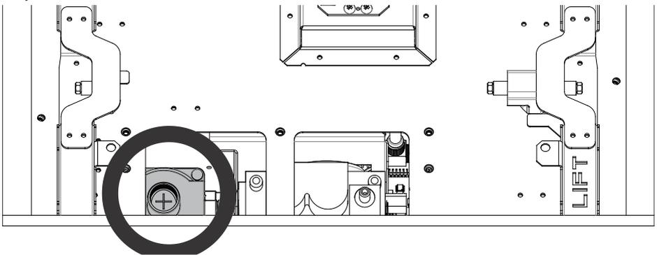
Once the operating pressure—post regulator—is set, check the operating pressure at test point A or D (shown in the first diagram of this section).
