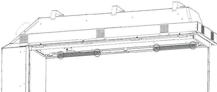
Once done, remove the 3 screws from the top side glass retainer, then loosen the screws on the bottom glass retainer (shown shaded in the diagram below). Carefully remove the glass panel from the firebox by tilting the top out first.
