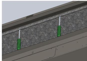
Remove the back glass panel by removing the 4 screws (circled below) in the two top retainers (shaded below). The glass will lift up and then swing out from the bottom.
