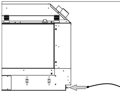
Two network cable access points are available: the primary connection is on the bottom of the RH outer face of the appliance for connecting permanently to the buildings' router; the secondary connection point is located where the AUX button is (shown in section E8 on page 30) for service technicians to access when the main connection method has not been used and has become inaccessible.
