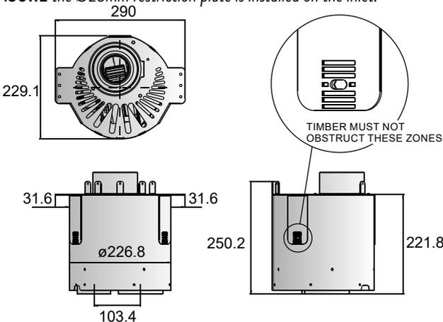
The UVP-Internal kit is intended for use within an accessible roof space or 'chimney' construction. **Service access must be provided.**
