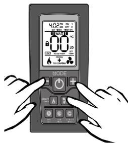
3. Press and hold the MINUS button until the two large temperature digits reading “00” start to flash slowly. Release the MINUS button. The remote control is now ready to be linked to the fire.
