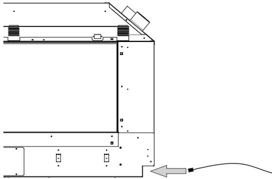
**If you do not connect the powerflue electrical cable to both the fireplace and the powerflue, this will result in an error when the fireplace is turned on.
