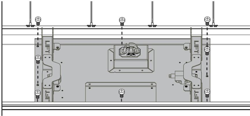
Remove 'engine' by lifting up and to the right. This is still connected internally to the gas hose and power cables.
