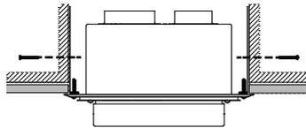
Attach the  $\varnothing 100\text{mm}$  and  $\varnothing 75\text{mm}$  flexible aluminium flues to the spigots on the rear of the horizontal powerflue wall terminal using the hose band clamps supplied. Plug the powerflue electrical cable into the back of the horizontal powerflue wall terminal.
