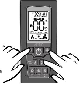
Whilst in test mode, press and hold the "ACTIVATE TIMER" and "FAN BOOST" buttons for 4 seconds to access the gas valve settings. The appliance will automatically turn on while in this mode.
