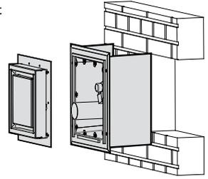
Fit the horizontal powerflue wall terminal into the hole and fix in place, making sure the installation is sealed appropriately to prevent the ingress of water from outside the wall cladding. Take notice of the label on the termination which shows the correct orientation of the terminal.
