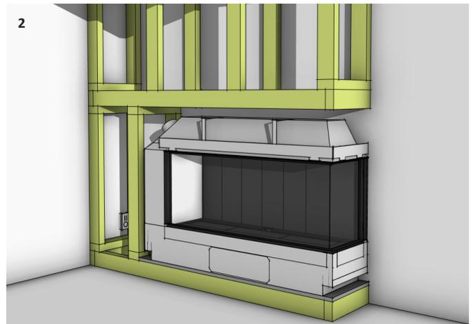
Install the appliance into the preformed cavity opening and secure it to the base. Ensure the fireplace is flush with the framework. Provide mains power connection and an accessible isolation switch.
