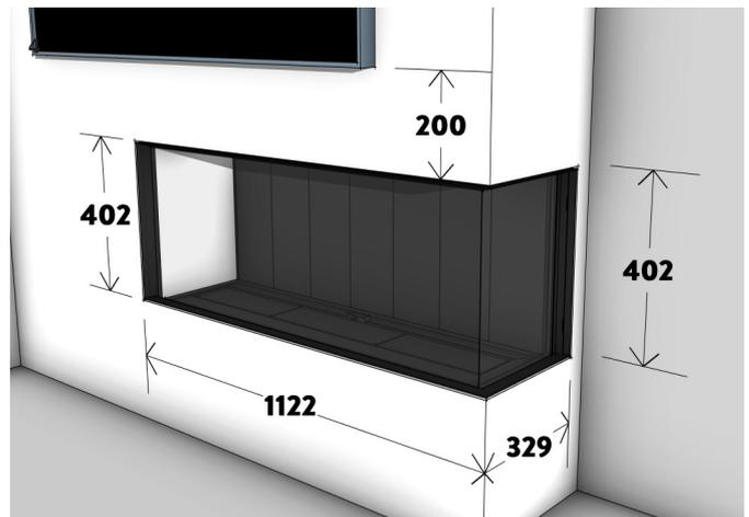
Attach wall linings to the framework and fireplace, maintaining a 3mm gap from the fireplace trim. Follow the provided wall lining cutout dimensions above for 20mm wall linings. Complete the project by adding additional finishes or fixtures.
