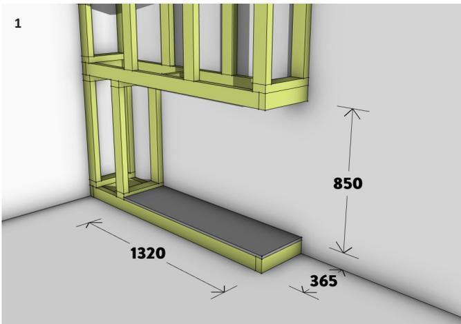
Build the chimney framework with consideration to flue pathways and meet the minimum fireplace opening requirements (1320mm W x 850mm H x 365mm D). Ensure a continuous base for the fireplace.
