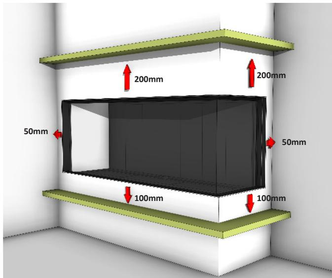
Ensure all clearances are met to any combustible or heat sensitive materials in front, above, to the side, or below the fireplace viewing area. Following these clearances, will allow the use of standard building materials, whether combustible or non-combustible. It is recommended to keep furnishings at least **1m** from the front of the fireplace.
