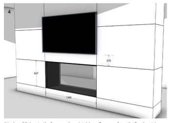
Attach wall linings to the framework, maintaining a 3mm gap from the fireplace trim. Follow the provided wall lining cutout dimensions above.
