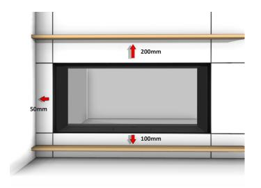
Ensure all clearances are met to any combustible or heat sensitive materials in front, above, to the side, or below the fireplace viewing area. Following these clearances, will allow the use of standard building materials, whether combustible or noncombustible. To reduce these clearances, use non-combustible materials.
