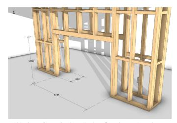
Build the chimney framework with consideration to flue pathways and meet the minimum fireplace opening requirement. Ensure a continuous base for the fireplace.
