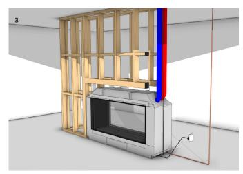
Connect flue pipes to the fireplace and create the flue pathway to the terminal. Connect Powerflue electrical cable at both ends.
