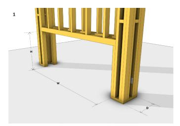
Build the chimney framework with consideration to flue pathways and meet the minimum fireplace opening requirements for a single sided installation (2087mm W x 850mm H x 350mm D). Ensure a continuous base for the fireplace.
