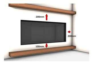
Install in accordance with AS/NZS 5601.1 and *KB1650 Install Manual*.
