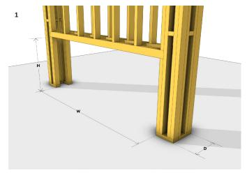
Build the chimney framework with consideration to flue pathways and meet the minimum fireplace opening requirements for a single sided installation (2418mm W x 928mm H x 350mm D). Ensure a continuous base for the fireplace.
