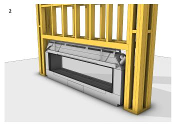
Install the appliance into the preformed cavity opening and secure it to the base. Ensure the fireplace is flush with the framework.
