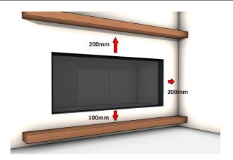
A hearth is not necessary, but if used, a combustible hearth must be at least **100mm** below the glass viewing area or made entirely of non-combustible materials.
