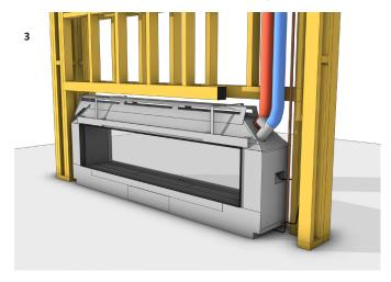
Install electrical, network connections, and gas supply. Connect flue pipes to the fireplace and create the flue pathway to the terminal. Connect Powerflue electrical cable at both ends.
