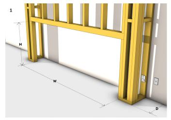
Build the chimney framework with consideration to flue pathways and meet the minimum fireplace opening requirements for a single sided installation (2418mm W x 928mm H x 365mm D). Ensure a continuous base for the fireplace.
