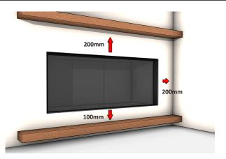
Install in accordance with AS/NZS 5601.1 and *KB1400 Install Manual*.
