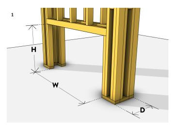
Build the chimney framework with consideration to flue pathways and meet the minimum fireplace opening requirements for a single sided installation (1500mm W x 850mm H x 350mm D). Ensure a continuous base for the fireplace.
