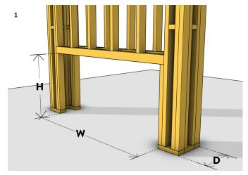
Build the chimney framework with consideration to flue pathways and meet the minimum fireplace opening requirements for a single sided installation (1793mm W x 850mm H x 350mm D). Ensure a continuous base for the fireplace.
