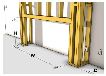
Build the chimney framework with consideration to flue pathways and meet the minimum fireplace opening requirements for a single sided installation (1793mm W x 850mm H x 365mm D). Ensure a continuous base for the fireplace.
