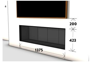
Attach wall linings to the framework and fireplace, maintaining a 5mm gap from the fireplace trim. Follow the provided wall lining cutout dimensions above for 10mm wall linings. Complete the project by adding additional finishes or fixtures.
