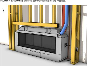
Install electrical, network connections, and gas supply. Connect flue pipes to the fireplace and create the flue pathway to the terminal. Connect Powerflue electrical cable at both ends.
