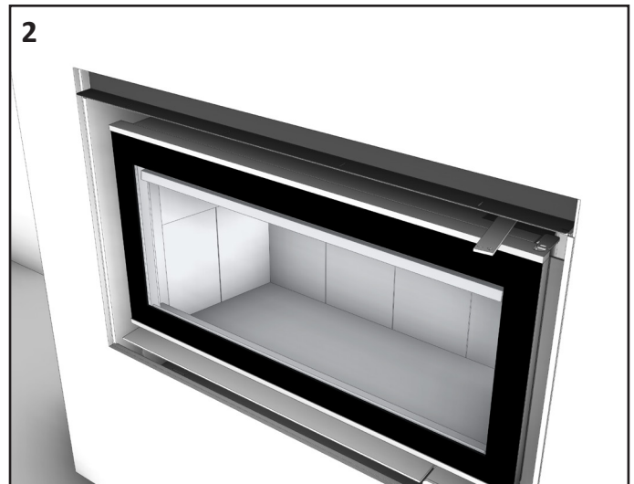
Align the fascia closure bracket, by pulling forward to have the up-stand in line with the ZCK or the back of the wall lining.
